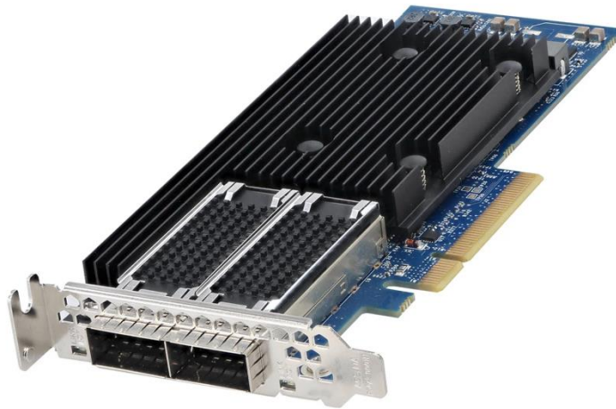
Figure 3: P4 SmartNIC - Netronome Agilio CX25
